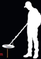
When you press the automatic calibration option, the user will see an instruction interface asking him to raise the dial a distance of 35 cm from the surface of the earth and then press the OK button to ask him to lower the search coil to a height of 10 cm. We notice an increase in the percentage of the indicator with a beep at this height.
