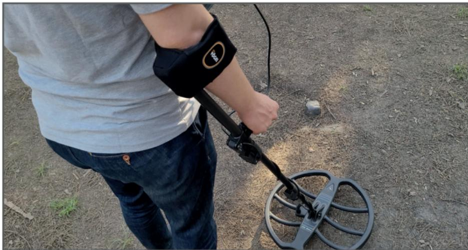
In this type of search, the user can activate the pointer option, which expresses the position of the target in relation to the disk, by pressing the Pinpoint button. When enabled, the discrimination pattern is temporarily disabled so that the device detects all targets. If the target is below the middle of the disc, the signal is maximum in the search area and decreases towards the edge of the disc.
