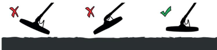
Wiping should be done by keeping the search coil parallel to the soil surface while avoiding excessive rubbing of the coil on the floor as shown in the figure.
