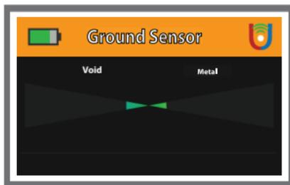
In case of metal target in the search are the indicator will show a high values in the high range of the display .
