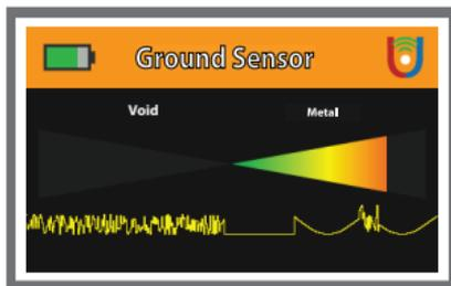
In this case the existing target is void and the interactive indicator with high values of blue according to the received signals and the target size in the search area
