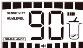
The screen displays 90 values, and the words GR-BALANCE light up to enter the automatic balance state
