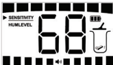
The minimum sensitivity level is 1 and the maximum sensitivity level is 99. The current screen display sensitivity is 68.
